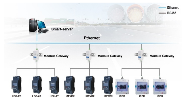
(485 MODBUS converter to Ethernet)
